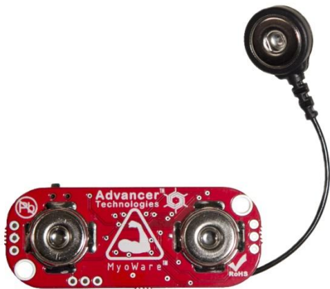
Figura 14.1: Sensor EMG de Advancer technologies.
